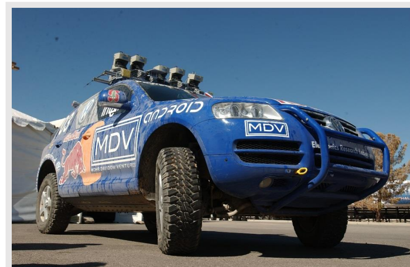
2005 DARPA Grand Challenge winner STANLEY performed SLAM as part of its autonomous driving system.
